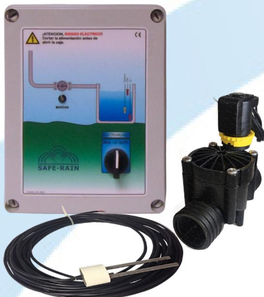
System that automatically controls the minimum and maximum water levels of architectural fountains with two electrodes, one for the minimum level and the other for the maximum level. When the minimum water level is reached, the solenoid valve connected to the sensor is opened. It closes automatically when the maximum level is reached.
